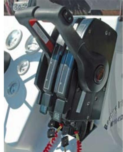
LEFT: Flares and other safety equipment can be easily accessed should an accident occur. CENTRE: The steering wheel is well positioned, giving the skipper good forward visibility. RIGHT: Each outboard has its own throttle and trim and tilt button.
